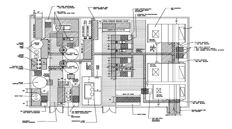
FIGURE 1 – SAMPLE MECHANICAL ROOM LAYOUT
