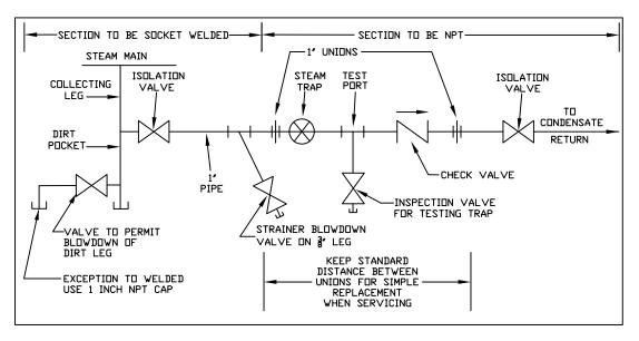
ALL 1" PIPE AND PIPE NIPPLES TO BE SCH. 80 SEAMLESS PIPE ALL 1" Y STRAINERS 300# SOCKET WELD ALL (4) 1" GATE VALVES TO BE 600# SOCKET WELD VOGT GATE VALVES CHECK VALVES 600# VOGT NPT 300# UNIONS-NPT - 1000# 90°EL'S NPT
